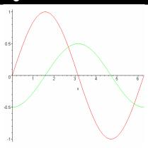
Here the red curve is current and the green curve is induced voltage. As you can see, the induced voltage lags the current by 90 degrees or the current leads the induced voltage by 90 degrees.
