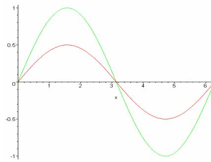
The current is represented by the green curve and the magnetic field strength is represented by the red curve. Note that the magnetic field is in phase with the alternating current.
