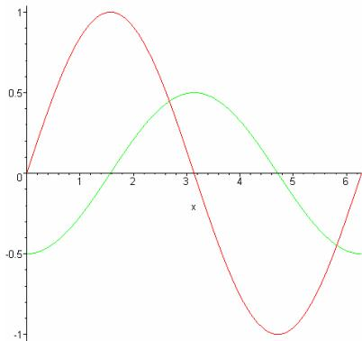
Here the red curve is current and the green curve is induced voltage. As you can see, the induced voltage lags the current by 90 degrees or the current leads the induced voltage by 90 degrees.
