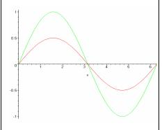
The current is represented by the green curve and the magnetic field strength is represented by the red curve. Note that the magnetic field is in phase with alternating the current.
