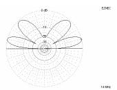
Notice that we now have two lobes, one at a low angle of radiation and the other at a higher angle of radiation. The lower lobe has an angle of radiation of about 14 degrees and will provide communication at a greater distance. The upper lobe has an angle of
