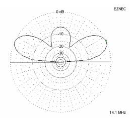
Here we are looking down the end of a dipole cut for 14.1 MHz.
