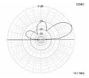
We are looking into the side of the array with the reflector on the left side and the driven element on the right side. The major lobe of the radiation pattern is to the right, away from the reflector, and the smaller (minor) lobe is to the left. On a single dipole we would have a pattern that would appear as follows:
