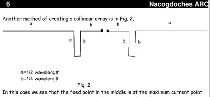
of a half wave length dipole therefore we have three half wavelength dipoles in phase. One reason for considering this type of antenna is to have lower impedance at the feed point of the antenna. The impedance at the feed point in Fig. 2 is in the neighborhood of  $300 \Omega$ , therefore, it has a reasonable match to  $300 \Omega$  transmission line.
