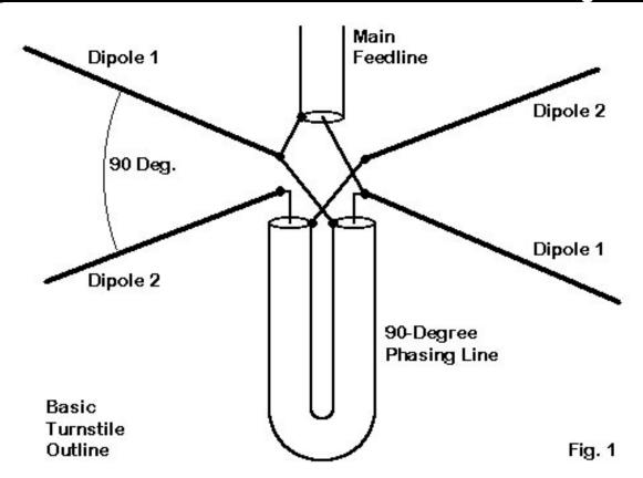
Since the impedance of a center fed dipole is around 70 ohms, then the 90-degree phasing loop can be made from RG-59 coax and should be  $\frac{1}{4}$  wavelength long. These dipoles are connected in parallel; therefore the impedances will combine like parallel resistances using the familiar formula
