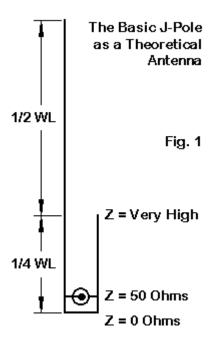
The vertical radiator is an electrical half wavelength and the matching stub is an electrical quarter wavelength parallel conductor. The feed point is moved up or down between the matching stub conductor and the main vertical element until the impedance is approximately 50  $\Omega$ . The electrical lengths of both the vertical radiator and the matching stub depend on the diameter of the conductor used in the
