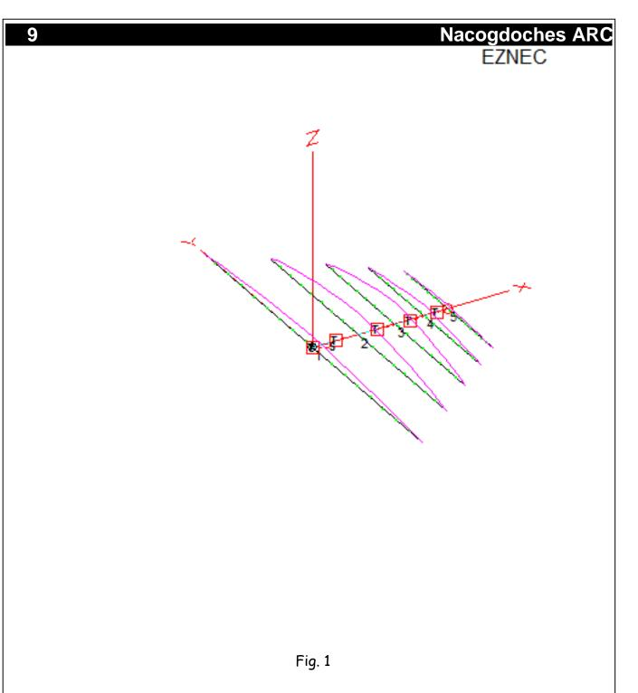
The five dipoles are labeled 1 through 5 and the pink curves represent current distribution on the elements. Remember, these elements are all driven using the phase shift technique described in the previous article.
